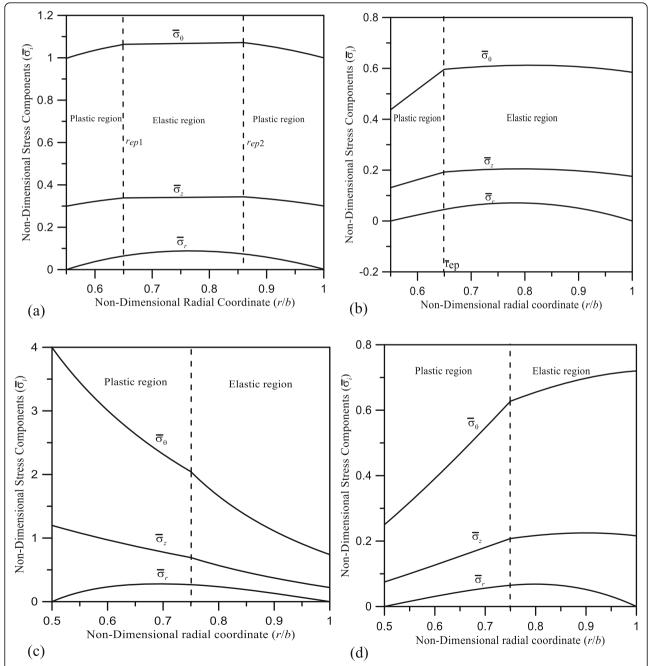
**Fig. 6** Stress distribution for (**a**)  $n_E = 1.3826$ ,  $n_P = n_o = 0$ . Yields from inside and outside  $(\overline{h} = 0.55, \Omega = 1.307)$ , (**b**)  $n_E = n_P = n_o = 1.3826$ ,  $\overline{h} = 0.55$  and  $r_{\rm ep} = 0.65(\Omega = 1.1999)$  yields from inside, (**c**)  $n_E = n_P = n_o = -2$ , and (**d**)  $n_E = n_P = n_o = 2$
