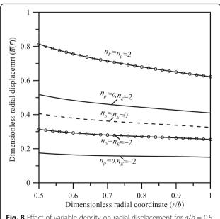
Fig. 8 Effect of variable density on radial displacement for a/b = 0.5
