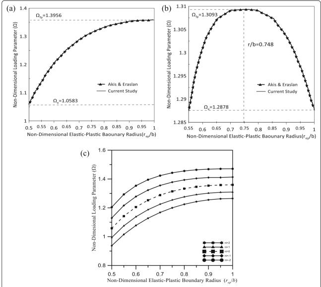
**Fig. 4** NLP plotted in different non-dimensional elasto-plastic boundary radius for (**a**) different  $n_i$ S, (**b**, **c**)  $n_E = 1.3826$ ,  $n_\rho = n_\sigma$ , comparing Akis results (Duc, 2016b) in different modulus of elasticity
