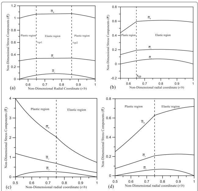
**Fig. 7** Stress distribution for (**a**)  $n_E = 1.3826$ ,  $n_P = n_o = 0$ . Yields from inside and outside  $(\overline{h} = 0.55, \Omega = 1.307)$ , (**b**)  $n_E = n_P = n_o = 1.3826$ ,  $\overline{h} = 0.55$  and  $r_{\rm ep} = 0.65$  (Ω = 1.19999) yields from inside, (**c**)  $n_E = n_P = n_o = -2$ , and (**d**)  $n_E = n_P = n_o = 2$
