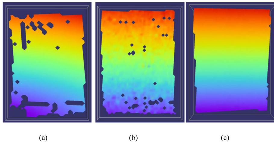
**Fig. 5** Comparison between the resultant displacement fields: **a** spray painted, **b** hand-marked and **c** CNC marked surface speckle patterns
