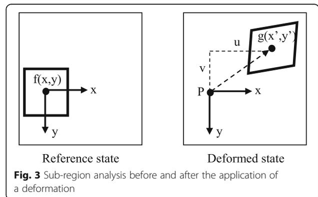
Fig. 3 Sub-region analysis before and after the application of a deformation
