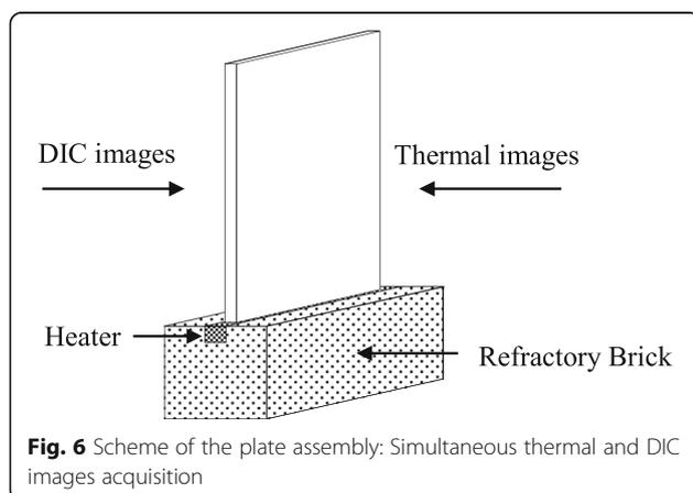
**Fig. 6** Scheme of the plate assembly: Simultaneous thermal and DIC images acquisition
