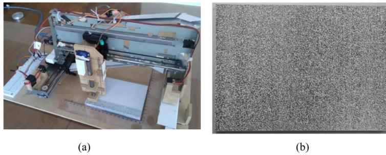
**Fig. 4 a** CNC marking device prototype marking a surface painted white. **b** Resultant printed speckle pattern with 40% of the total area covered with black speckles
