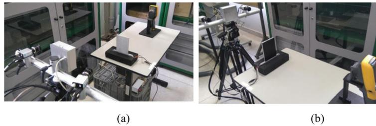
**Fig. 7** Experimental assembly: **a** DIC system point of view, **b** thermal imager point of view
