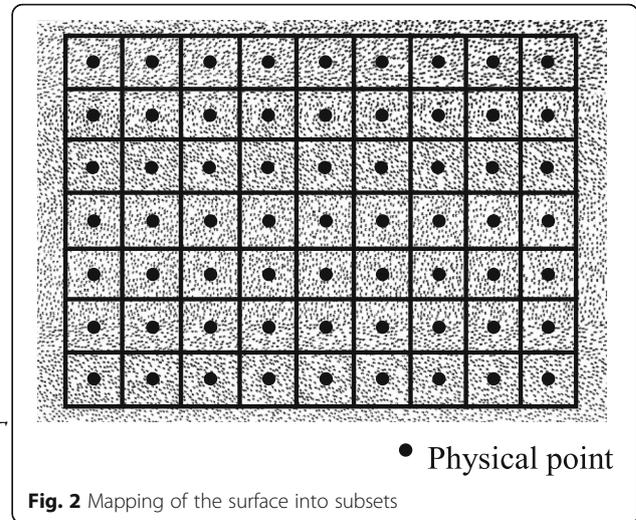
Fig. 2 Mapping of the surface into subsets
