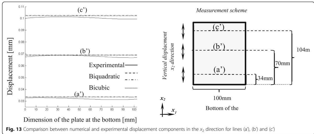
**Fig. 13** Comparison between numerical and experimental displacement components in the  $x_2$  direction for lines (a'), (b') and (c')
